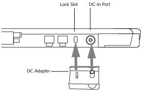
Figure 1. Attaching the DC Adapter
